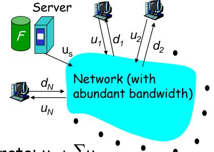
$$d_{P2P} = \max \{ F/u_s, F/\min(d_i), NF/(u_s + \Sigma u_i) \}$$
