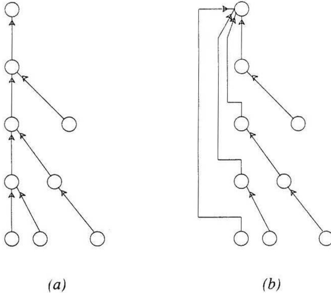
**Figure 4.17** Path compression: (a) Before. (b) After.
