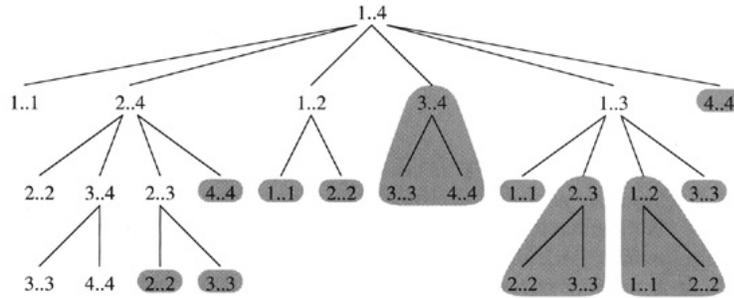
**Figure 15.5** The recursion tree for the computation of `RECURSIVE-MATRIX-CHAIN(p, 1, 4)`. Each node contains the parameters  $i$  and  $j$ . The computations performed in a shaded subtree are replaced by a single table lookup in `MEMOIZED-MATRIX-CHAIN(p, 1, 4)`.
