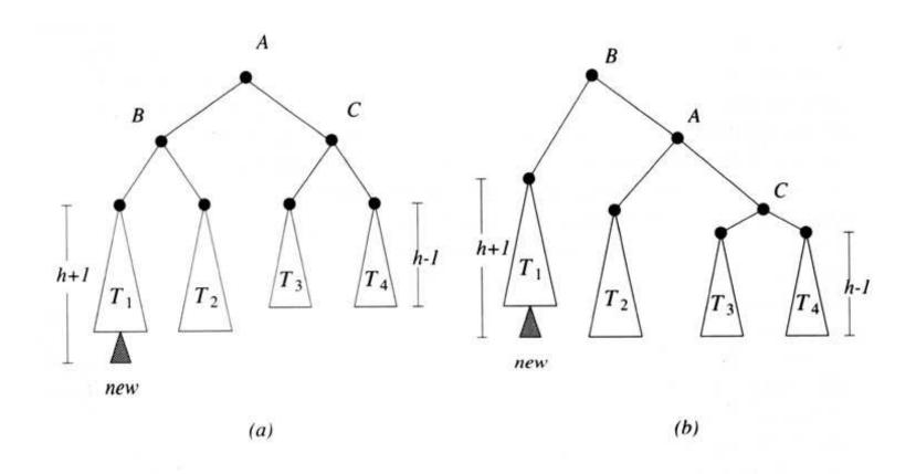
Figure 4.14 A single rotation: (a) Before. (b) After.
