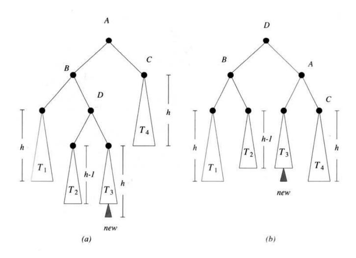
Figure 4.15 A double rotation: (a) Before. (b) After.
