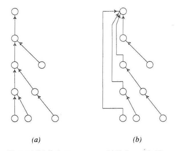
Figure 4.17 Path compression: (a) Before. (b) After.
