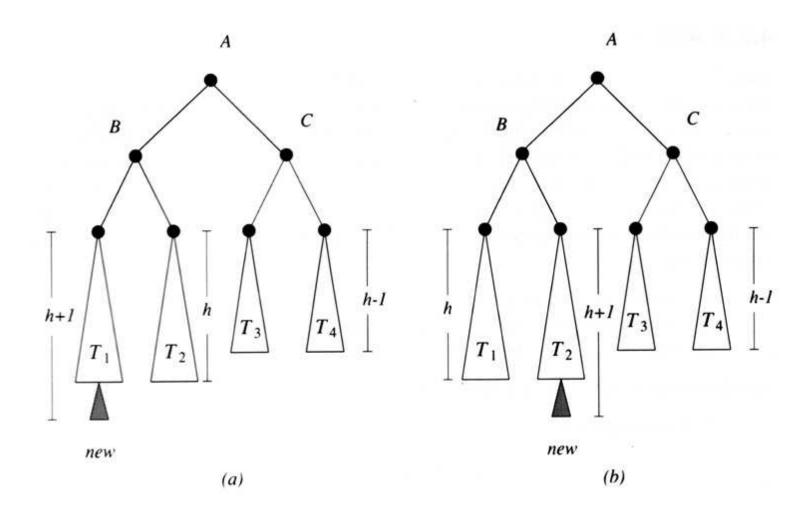
Figure 4.13 Insertions that invalidate the AVL property.
