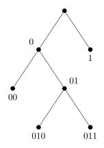
Figure: The tree representation of encoding. Source: redrawn from [Manber 1989, Figure 6.17].
