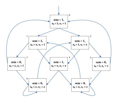
Use the symbolic CTL model checking algorithm in [CGP; Chapter 6] to compute the states that satisfy the CTL formula  $\mathbf{AG}((s_0=e)\to\mathbf{AF}(s_0=c))$ .
