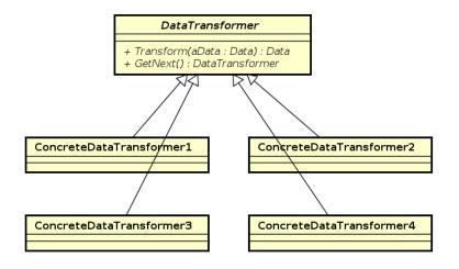
Each concrete DataTransformer may decide what transformation to apply after its Transform() is finished. For example, ConcreteDataTransformation1 may decide the next transformation to be ConcreteDataTransformation 2, 3 or 4 depending on the result of its transformation:
