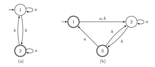
11. (Exercise 1.24; 5 points) A finite-state transducer (FST) is a type of deterministic finite automaton whose output is a string rather than accept or reject. The following are state diagrams of finite state transducers  $T_1$  and  $T_2$ .
