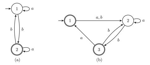
8. (Exercise 1.24; 10 points) A finite-state transducer (FST) is a type of deterministic finite automaton whose output is a string rather than accept or reject. The following are state diagrams of finite state transducers  $T_1$  and  $T_2$ .
