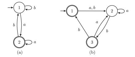
7. (Exercise 1.24; 10 points) A finite-state transducer (FST) is a type of deterministic finite automaton whose output is a string rather than accept or reject. The following are state diagrams of finite state transducers  $T_1$  and  $T_2$ .
