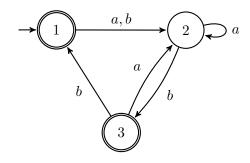
7. (Exercise 1.24 adapted; 10 points) A finite-state transducer (FST) is a type of deterministic finite automaton whose output is a string rather than accept or reject. The following are state diagrams of finite state transducers  $T_1$  and  $T_2$ .
